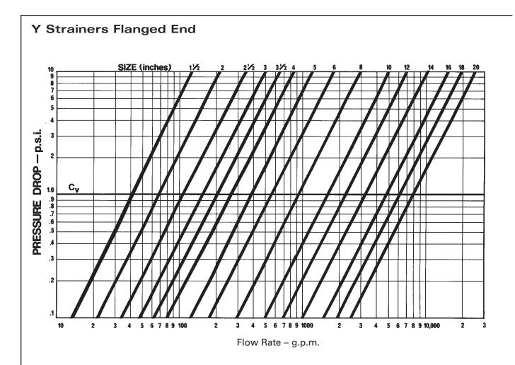
Above based on the flow of clean water through .033" - ¼" perforated metal screens. Consult our Engineering Department for pressure drop information on steam, gases or viscous fluids. See Theoretical Pressure Drop Curves for Screen Clogging In the Technical Data Section for multiplying factors for clogged screens.
