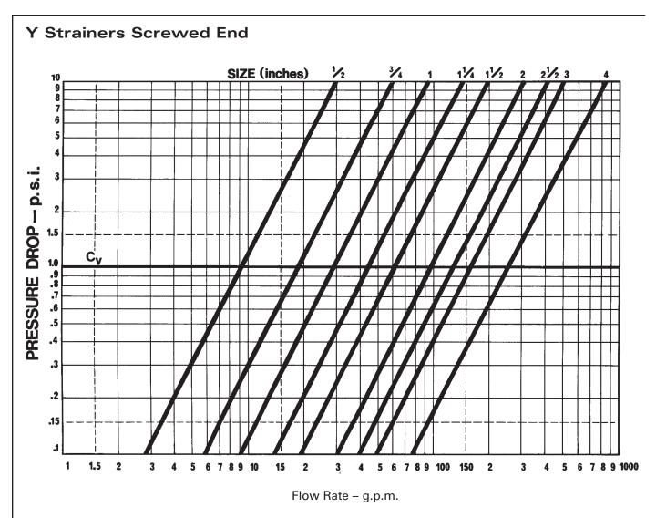
Above based on the flow of clean water through .033" - ¼" perforated metal screens. Consult our Engineering Department for pressure drop information on steam, gases or viscous fluids. See Theoretical Pressure Drop Curves for Screen Clogging In the Technical Data Section for multiplying factors for clogged screens.
