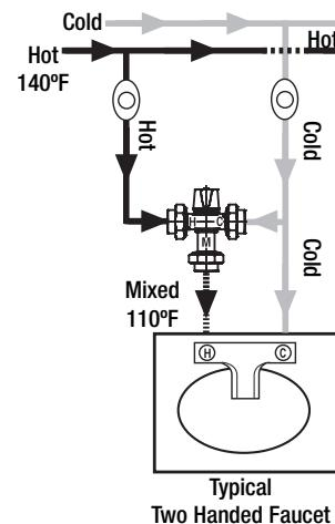
to the hot side of a two-supply valve (faucet or roman tub fitting) and allows further tempering (w/cold) downstream. It can be adjusted by the user. Common applications are sinks and whirlpool tubs; hence the temperature variance or control is not as tight ( $\pm 7^{\circ}\text{F}$ ) as required for a shower application.
