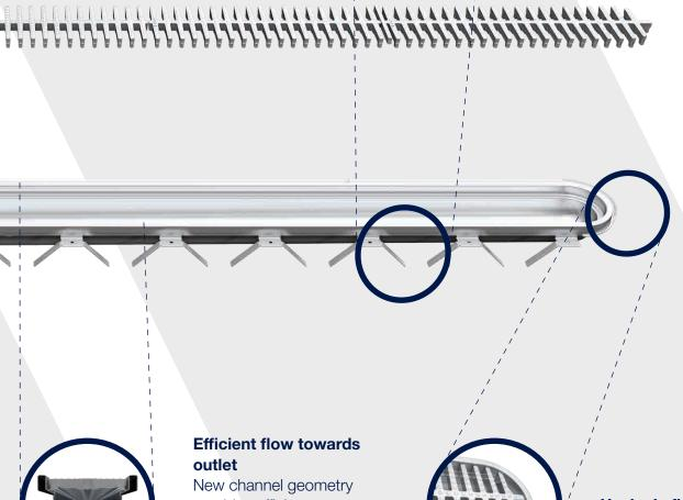
New channel geometry provides efficient transportation to outlet area, keeping channels empty and clean, even during minimal water flow.
