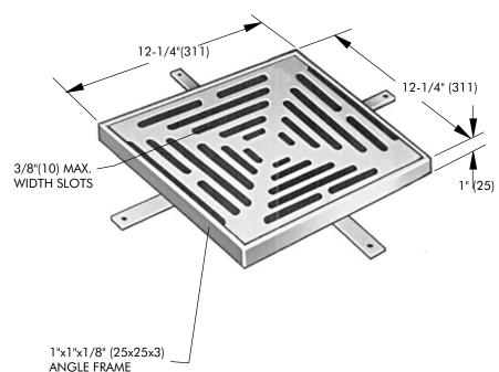
Order Code: TD-900-Ex. TD-900-B2-4-1 Pieces (Select One) Suffix Description 1 Piece 2 Piece В3 3 Piece Specify x: Grate (Select One) Suffix Description Ductile Iron Grate w/ Steel Frame -4-1 Ductile Iron Grate w/ NB Veneer & Frame Ductile Iron Grate w/ Stainless Steel Veneer & Frame All Solid Stainless Steel Grate & Frame
