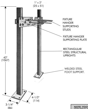
NOTE: FOOT SUPPORTS SHOULD BE SECURELY ANCHORED TO FLOOR WITH 1/2" BOLTS AND ANCHORS BY OTHERS.
