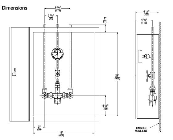
Note: Dimensions are shown ±1/2" Dimensions in parentheses are in mm
