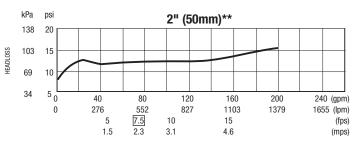
\*\* Metric Dimensions are nominal pipe diameter. This product is produced with NPT threaded end connections.
