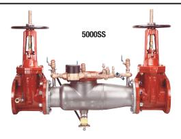
bottom mounted and supplied with a steel reinforced sensing hose. The assembly shall include two resilient shutoff valves and four ball type test cocks and a hydraulically balanced by-pass line. The bypass line shall include a meter, small diameter reduced pressure zone assembly and isolation valves. The bypass reduced pressure assembly shall have a single bolted on cover and top mounted test cocks. The assembly shall be an Ames Fire & Waterworks Series 5000SS.
