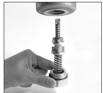
Remove body cap with wrench to service cold water poppet assembly.
