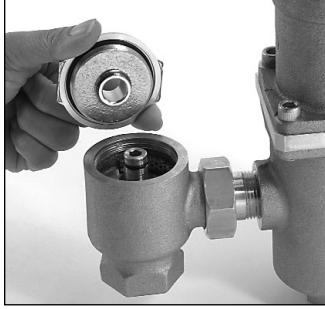
Remove bonnet with 2-1/4" (57mm) wrench for 3/4" NPT checks and 3" (76mm) for 1-1/4" NPT checks or use a 3/4" socket wrench.
