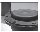
Line up diaphragm bolt holes with body flange bolt holes.
