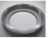
This will ensure that excess rubber will roll to the inside of the main guide when the holder assembly strokes, otherwise the diaphragm will crack and leak.
