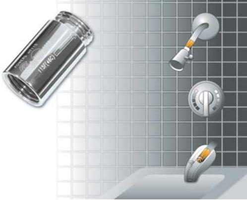
Quickly retrofit your shower, tub or lavatory applications with our ScaldStop high temperature shut-off valve. Water flow is reduced to a trickle if the temperature reaches 115°F. The valve simply threads onto an existing shower arm and is housed inside the tub spout itself. Both install in minutes without the need for special tools.
